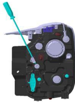
8 9 10 11 12 13 14 Fig. 5. Low and High-Beam Aim Adjusters Inside Class Vehicle Headlight 15 Assembly
