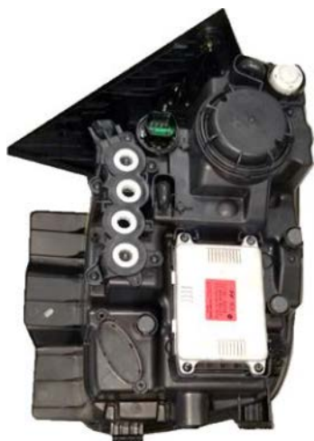
Fig. 4.2. Inside of Headlight Assembly with Circular Seal in Upper Right Corner
