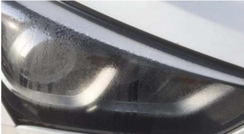
Fig. 3. Class Vehicle Headlight Assembly with Improper Moisture Intrusion
