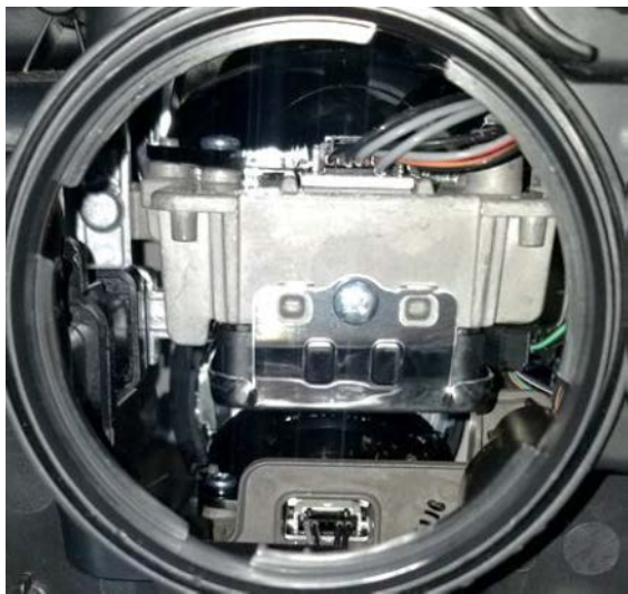
Fig. 4.3. Wiring and Headlight Connections Inside Circular Seal within Headlight Assembly
