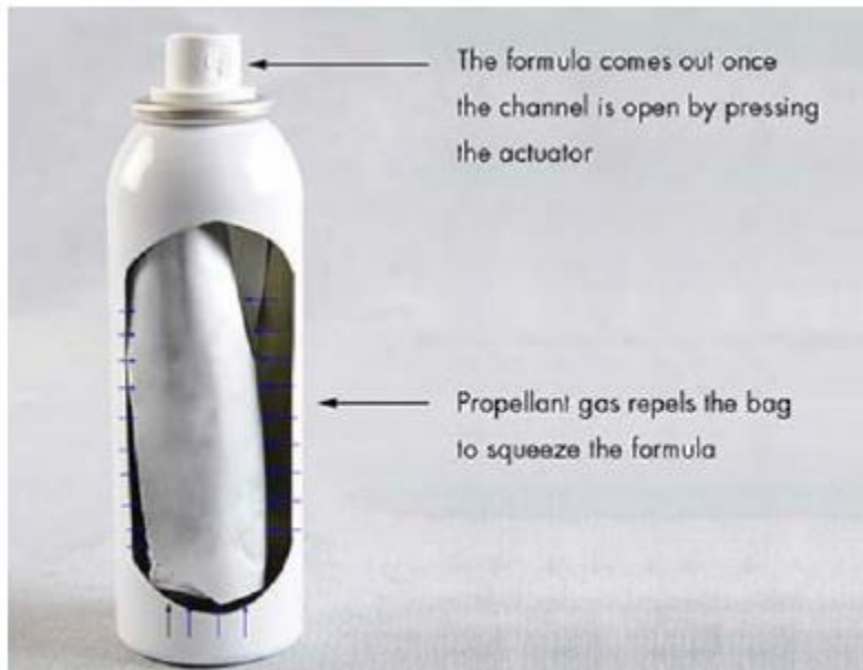
Figure 10: Visual of a BOV system.
