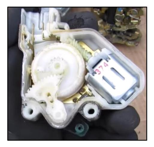
30. In the Class Vehicles, the sliding door fails to lock or unlock with the electronic controls, and often will not open—even manually. Failure to lock or unlock the sliding door with electronic controls or even manually is an indicator that the actuator is not functioning properly. Normally, a slight clunking sound or whirring sound can be heard when the locks are activated. If the sound of the actuator becomes weak or excessively noisy, it is a sign that the actuator may be failing. In
