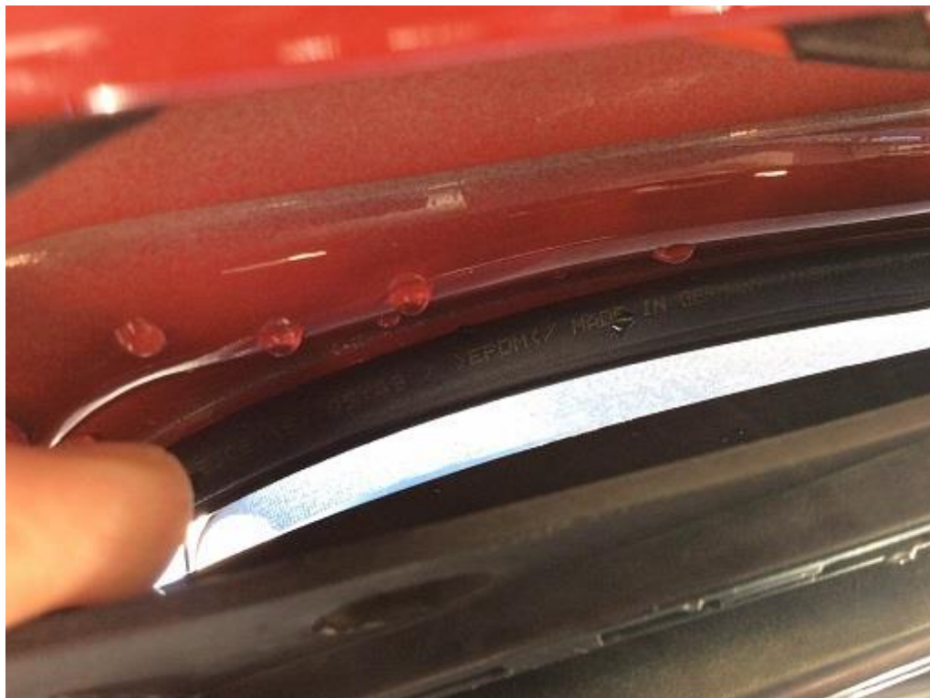
Figure 1: water leaking between sunroof frame and body
