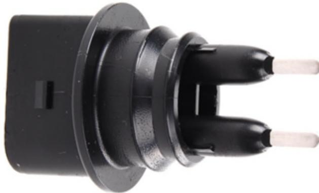
25. Electricity is conducted between these prongs only when they are immersed in the washer fluid. When the fluid level falls below the level of the prongs, an electrical charge does not pass, and the sensor triggers a warning light on the dashboard indicating that washer fluid is low.
