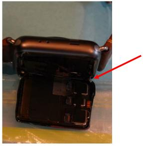
5. When a consumer's body contacts the sharp edge of the detached, shattered, or cracked screen, there is substantial and material risk of serious injury, including lacerations, cuts, abrasions, and other injuries.
