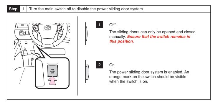
\*: The power function of the power back door will be disabled while the switch is in this position. The power back door can still be used manually.
