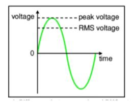
For most of the time, the wave is below the peak voltage, so peak voltage is not typically a helpful measure of its real effect. This is why the root mean square voltage, or RMS, is used. Similar to voltage, currents (such as sine waves) are calculated formulaically.<sup>7</sup>
