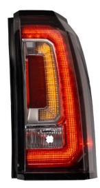
21. The tail lamp assembly includes tail lights that illuminate when the headlights are turned on to create visibility for drivers behind you during the night or adverse weather conditions. Just as the headlights make your vehicle visible to others on the opposite side of the road, the tail lights make your vehicle visible to cars behind you. The assembly also includes
