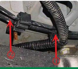
Move the wire harness retaining clip from the steel lines (1) to in front of the steel line support (2).
