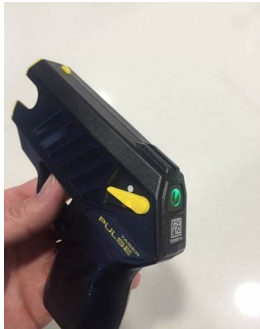
Figure 2: Showing Plaintiff's Actual Pulse CEW as Armed (Indicated by the Green Light) With the Safety Lever Not Even Halfway to the "Armed" Position. 4
