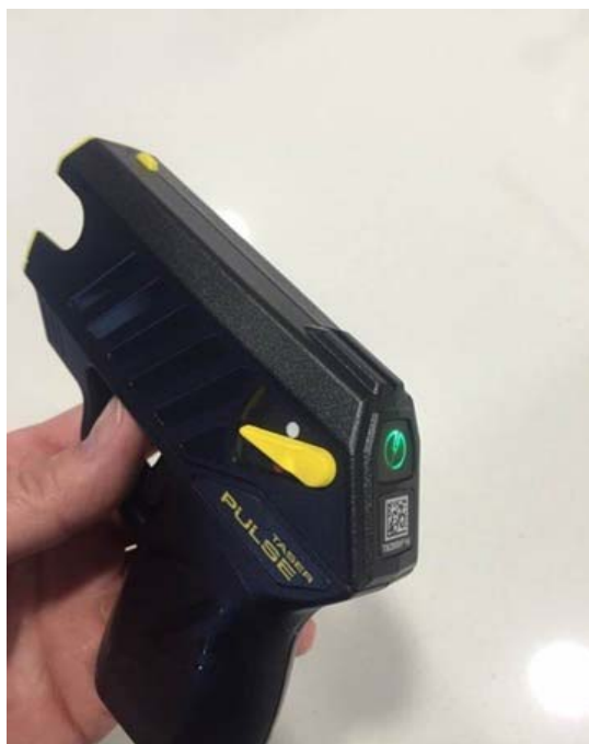
8 9 Figure 2: Showing Plaintiff’s Actual Pulse CEW as Armed (Indicated by the Green Light) 10 With the Safety Lever Not Even Halfway to the “Armed” Position. 4
