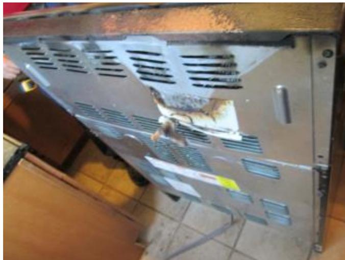
27. The Reichardts would not have purchased the electric range at issue had Electrolux disclosed that the range's electrical system contained the Defects at the point of sale. The Defects caused their Frigidaire electric oven range to overheat and catch fire. Because of the Defects, they did not receive the benefit of their bargain.
