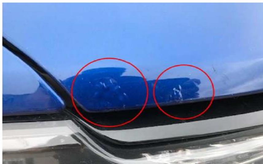
Fig. 1 Examples of Corrosion Along Leading Edges
