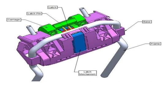
67. When a vehicle is involved in a rear-end collision, the device propels the face of the headrest forward by 40 millimeters and upwards by 30 millimeters, to meet the head as it
