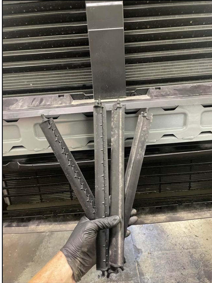
Figure 3: Image of four blinds removed from a Ford Maverick active grille shutter system as part of Ford’s “fix” for the Stall/Fire Risk Vehicles 11
