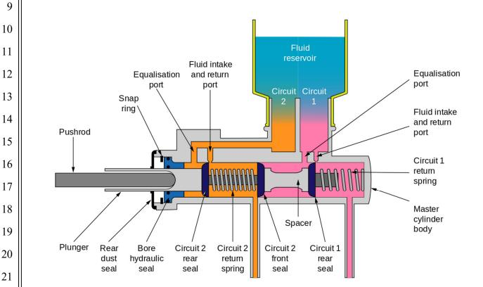
(a) In general, there are two separate hydraulic circuits in a master cylinder. Each circuit supplies pressure to the calipers at two wheels. Each circuit is hydraulically independent with the exception of drawing fluid from the reservoir when at rest;
