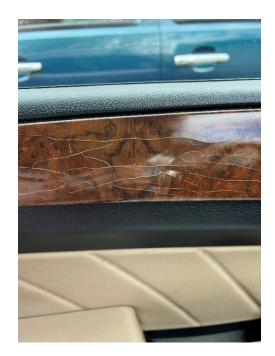
64. Ms. Monilaw's vehicle is just one of thousands of Putative Class Vehicles that have this defect in the interior trim that results in cracking of the interior Veneer Wood Trim.
