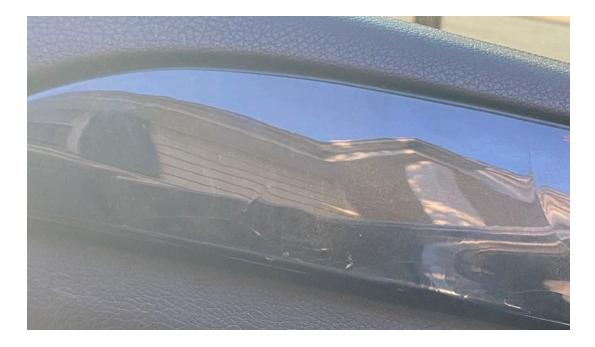
76. Ms. Burzes's vehicle is just one of thousands of Putative Class Vehicles that have the defect in the interior trim that results in cracking of the interior Veneer Wood Trim.
