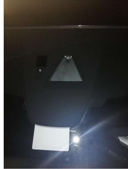
53. The FSC determines the conditions ahead of the vehicle while travelling at night and detects traffic lanes. The distance from which the FSC can detect objects depends on the surrounding conditions.
