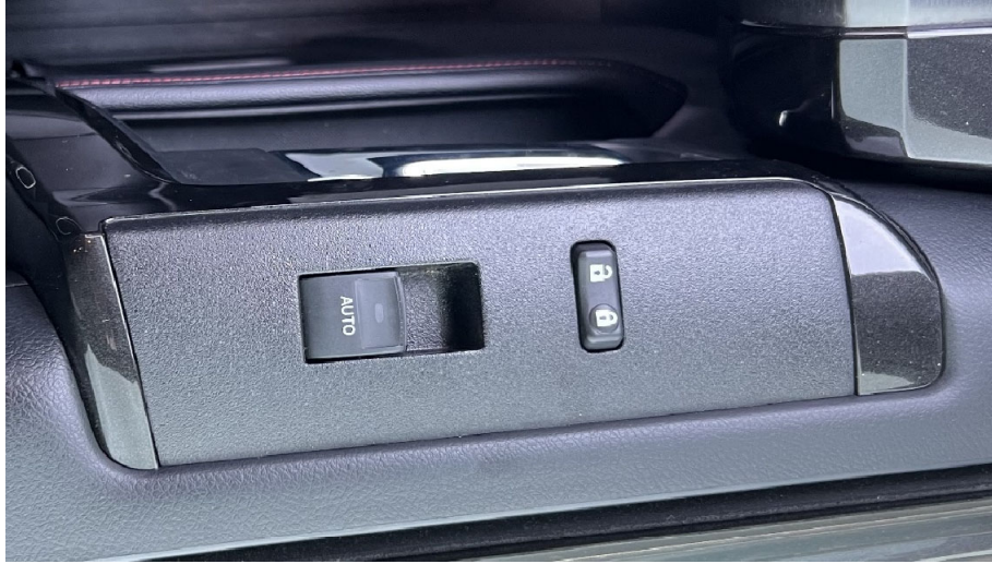
Toyota 4Runner Passenger Side Power Window and Door Lock Controls (Below)
