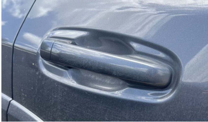
Rear Passenger Side Exterior Door Handle without Key Lock (Toyota 4Runner)
