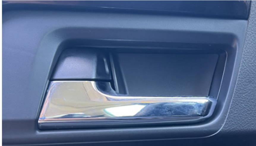
Flip-style interior door lock in the locked position (Toyota 4Runner)
