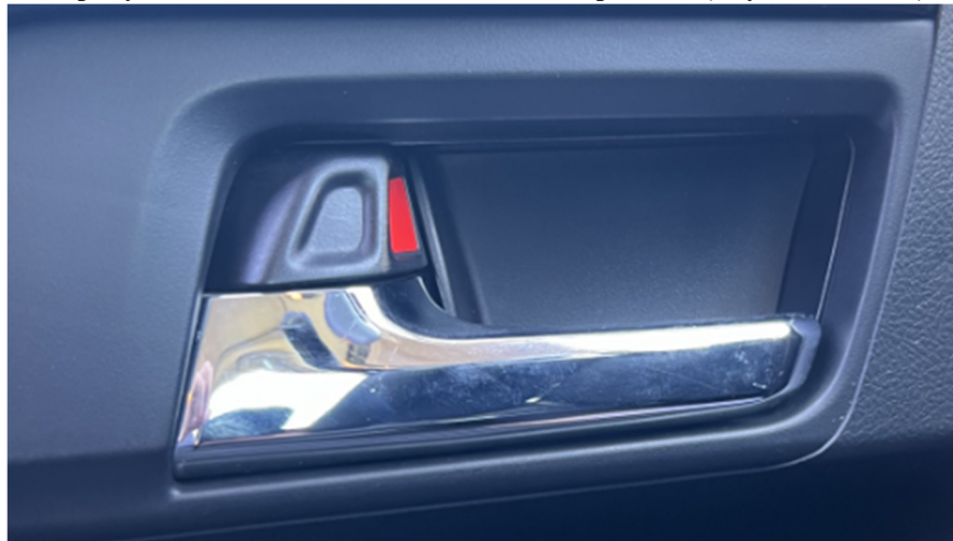
Flip-style interior door lock in the unlocked position (Toyota 4Runner)
