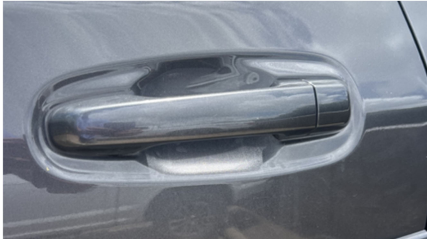
Rear Driver Side Exterior Door Handle without Key Lock (Toyota 4Runner)
