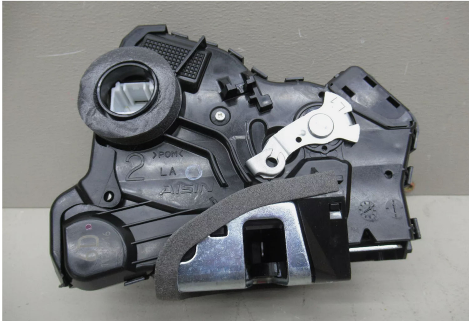
Part No. 69040-42250 Door Lock Actuator View #2 (Below)
