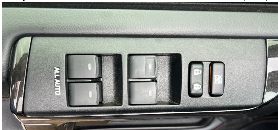
Toyota 4Runner Driver Side Power Window and Door Lock Controls (Below)
