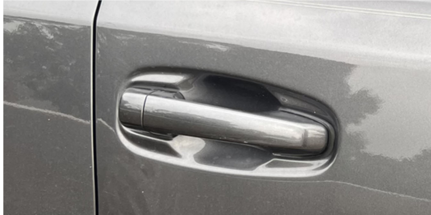
Rear Driver Side Exterior Door Handle without Key Lock (Toyota 4Runner)
