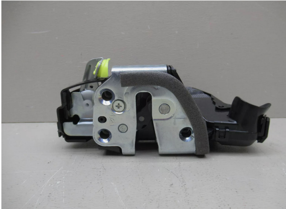
Internal Image of the Door Lock Actuator (Toyota 4Runner)
