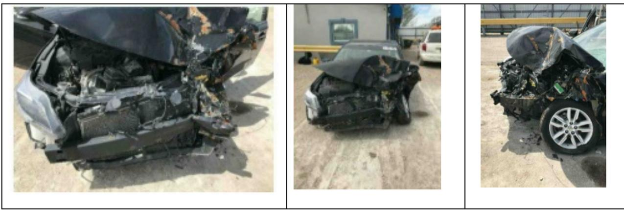
1043. On April 10, 2019, an inspector for Toyota USA inspected the wreckage of this vehicle. The EDR data recovered from the Avalon had no record of the crash. This was a sign of ASIC EOS.
