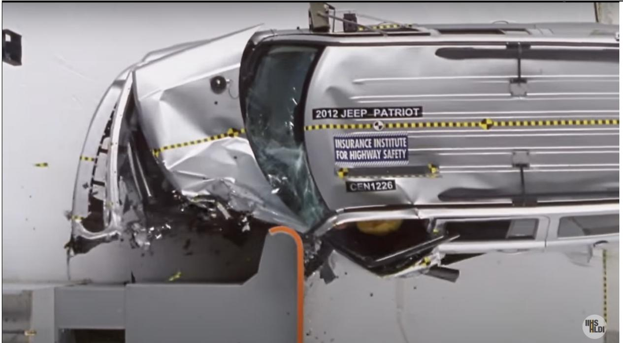
807. All of the airbags in the 2012 Jeep Patriot should have deployed given the severity of the crash into the rigid barrier.
