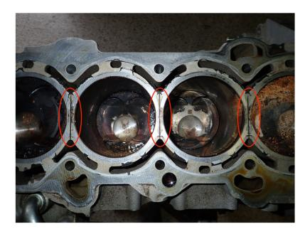
25. In a non-defective engine, liquid coolant is used to ensure that the engine does not overheat. The coolant circulates through a set path within the engine block and cylinder head, cooling the engine. The liquid gathers heat due to contact with the engine and then flows through a hose and into the radiator to cool back down. Once its temperature has lowered, the coolant returns to the engine, and continues to circulate.
