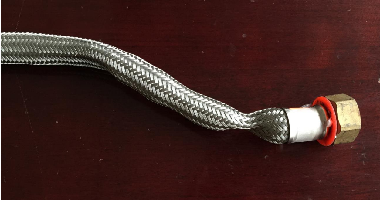
Figure 2 : Close-up View of Failed Line (at location of failure)
