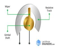
39. A potentiometer is connected to each joystick shaft, as well as the controller's circuit board and works as an electrical circuit. Each potentiometer consists of a curved, resistive track and a contact arm. Moving the contact arm increases or decreases the electrical current flowing through the circuit. The stick's physical position is translated into an electrical signal, which is then converted into a digital reading that can be read by the operating system.
