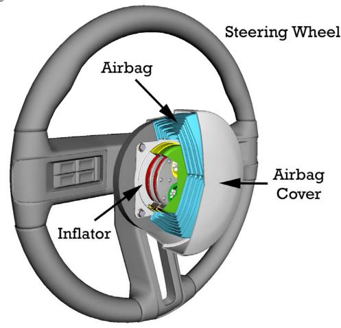
46. When it began manufacturing airbags in the 1980s, Takata used sodium azide as the propellant within its inflators. In the mid-1990s, Takata began using a different propellant called 5-aminotetrazole, in part due to toxicity issues associated with sodium azide.
