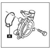
• Gaskets and pipe for high pressure fuel pump
