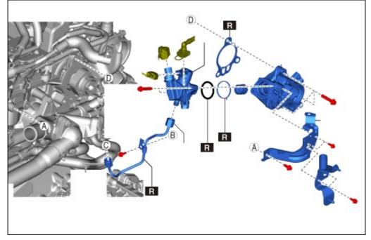
· Gasket and O-rings for water pipes and cylinder head gasket
