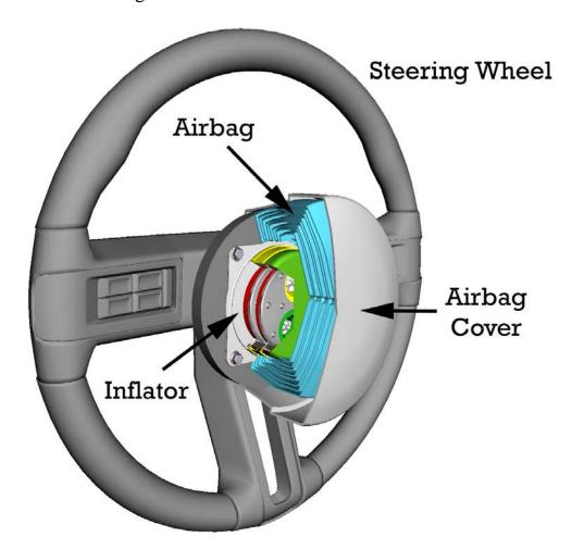
81. When it began manufacturing airbags in the 1980s, Takata used sodium azide as the propellant within its inflators. In the mid-1990s, Takata began using a different propellant called 5-aminotetrazole, in part due to toxicity issues associated with sodium azide.
