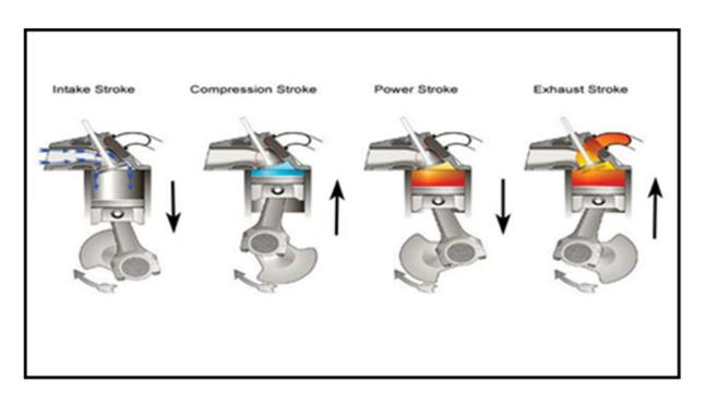
65. The engines in the Class Vehicles utilize fuel injectors mounted on the cylinder head, rather than on the intake manifold as in traditional engine applications. This fuel delivery method in the Class Vehicles is known as gasoline direct injection ("GDI") whereby fuel is injected at a very high pressure directly into the combustion chamber rather than through the intake manifold.
