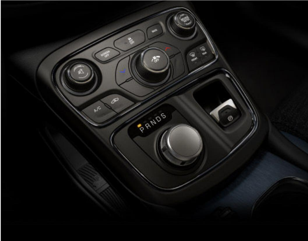
The above-pictured designs are superior to the E-shift System because they unambiguously link user input to mechanical results—i.e., they provide the tactile and visual feedback drivers expect. A driver simply has to turn the knob completely to the left or push a button to shift into Park. In the Defective Vehicles, however, a driver who presses the gearshift forward could land in either Neutral, Reverse, or Park.
