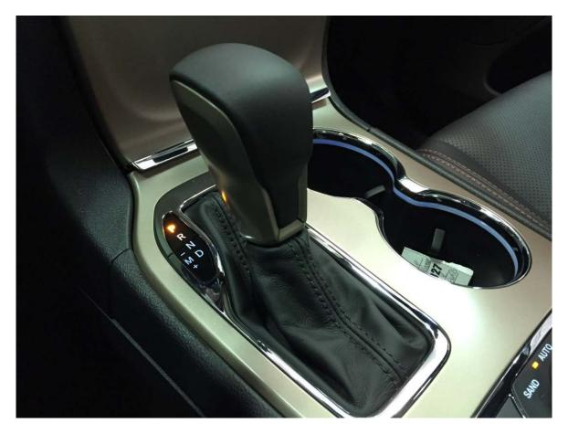
32. In contrast, a monostable shifter has a single central position that it snaps back to when the driver releases the shift knob. To shift gears, the driver depresses a button on the shift-
