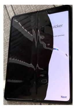
11. The Product is highly susceptible to screen damage including corrupted pixels, through microscopic particles getting under the protective film at the hinge, creating air pockets.
