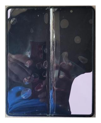
12. Even cold temperatures are capable of causing the screen protector to snap instead of bend, rendering the screen non-functional when the phone is unfolded.
