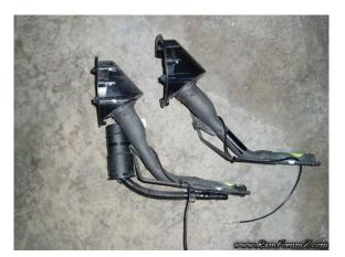
31. Other Ram owners have provided directions for another at-home remedy in which, instead of completely replacing the part, the angle of the defective filler neck is physically altered with a wire:
