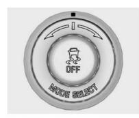
The PTM system contains five modes. These modes are selected by turning the Selective Ride Control/Performance Traction Management MODE SELECT knob on the center console. Scroll up or down through modes 1–5 by turning the MODE SELECT knob to the right or left. The following is a DIC display description and the recommended usage of each mode:
