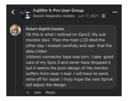
Ok this is what i noticed on Xpro3. My sub monitor dies. Then the main LCD died the other day. I looked carefully and saw that the data/video (ribbon) connector tape was torn. I take good care of my Xpro 3 and never have dropped it but it seems the poor design of the monitor suffers from wear n tear. I will have-to send mine off for repair. I truly hope the next Xpro4 will adjust the design.
