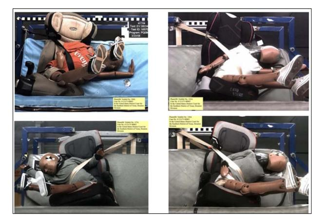
167. These images show the seat belt slipping off the dummy's shoulders and instead tightening around its abdomen and ribs. This kind of violent movement at high speed can cause serious damage to a child's internal organs, head, neck, and spine, including paralysis or death.
