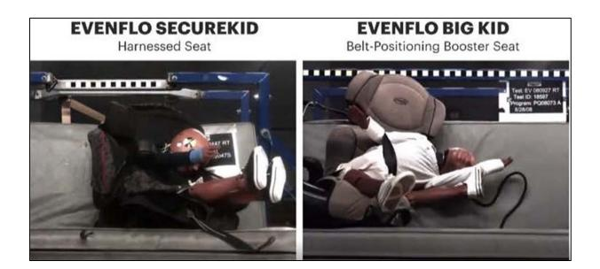
148. In the test of the SecureKid, the dummy's head and torso remained entirely within the seat's confines. By contrast, in the test of the Big Kid, the seat belt slipped off the dummy's shoulder, and the dummy's head and torso flailed far outside the seat.
