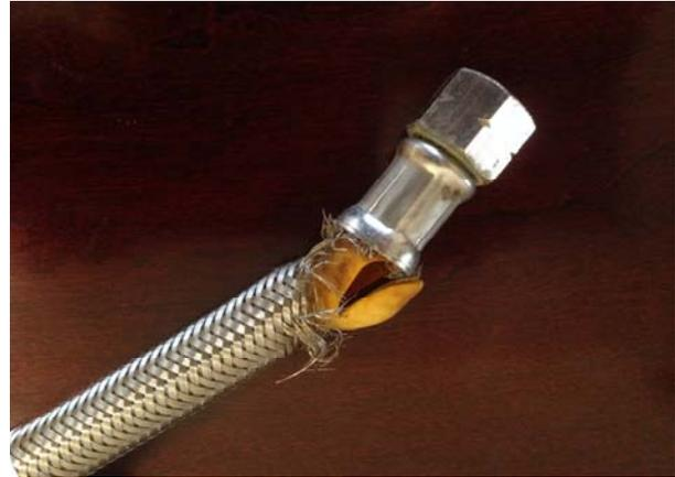
61. Chloride stress corrosion is a well-known and generally accepted phenomenon in the scientific community and in the plumbing industry. Fluidmaster knew or was reckless in not knowing that by selecting an inferior grade of stainless steel, combined with low-pressure inner rubber tubing, it was creating a product designed to fail. These defects were present at the time of manufacture and sale to Plaintiffs and the Class who had no knowledge of the defects.
