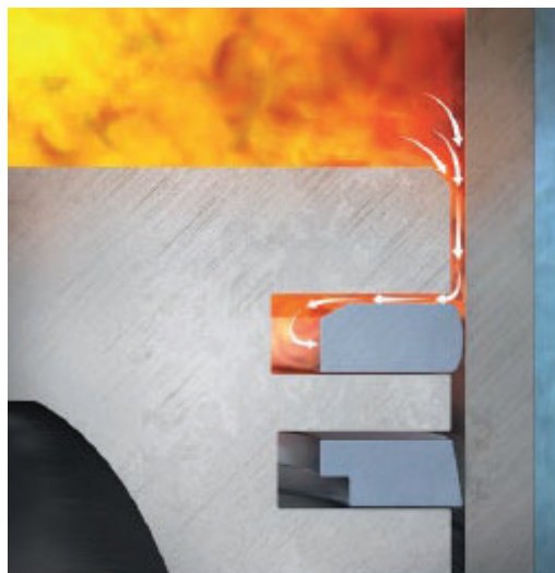
Sealing against combustion gases
