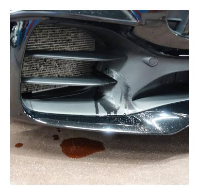
37. Other Class Vehicles, as evidenced by the photograph below, are equipped with "egg-crate" style guards that are insufficient to protect the aluminum radiators. These vehicles suffer from the same Inlet Defect as vehicles with no protective guards at all because the guards are insufficient to protect against rocks, pebbles and/or other road debris from entering and damage the Class Vehicles' aluminum radiators.
