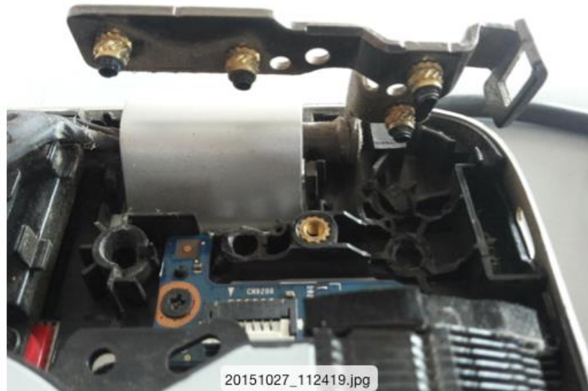
Fractured Plastic Anchors in 17" HP Envy 1
