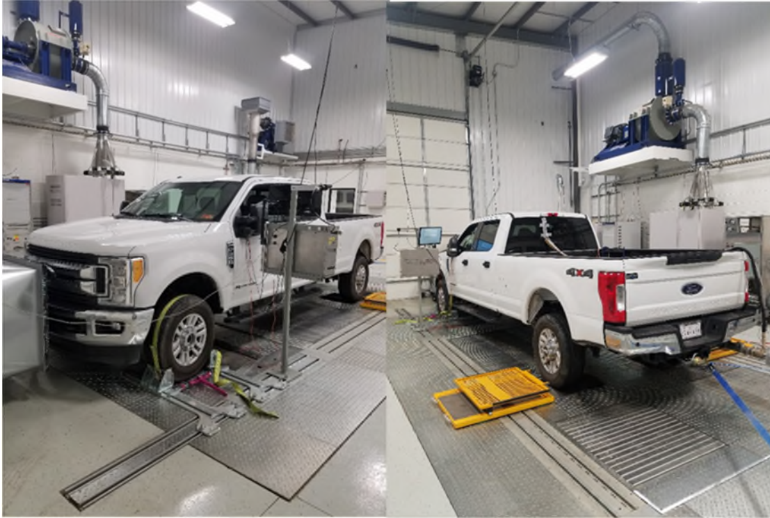
2017 Ford F350 during dynamometer testing
