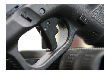
19. In addition to the Glock, other popular versions of striker-fired pistols come with external safety features such as a trigger safety toggle and/or a manual safety:
