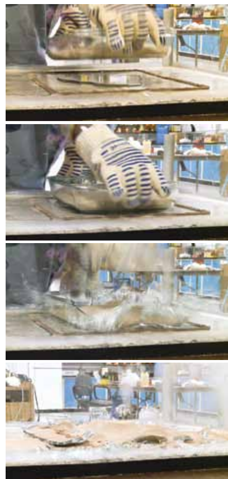
Figure 2. Heat test: Frames from video of tests conducted by Consumer Reports' shows bakeware made of soda lime silicate glass shattering after being heated in a 450°F degree oven and placed on a wet countertop.
