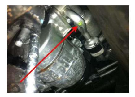
If the a/c line cracks, it may spray oil and refrigerant onto the a/c compressor, making the leak very hard to identify.
