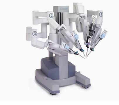
26. Doctors direct the surgery by manipulating controllers on the robot console, which allow for precision control of the robot arms and EndoWrist instruments. This allows the surgeon to specify movements on a scale that is at least an order of magnitude less than the surgeon's actual hand movements at the console. The image below shows a doctor manipulating the instruments:
