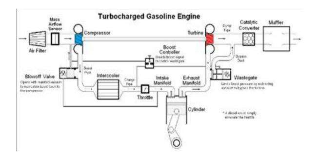
28. Turbochargers are a forced induction system that compresses air flowing into a vehicle's engine, allowing the engine to burn more fuel by forcing more air into the vehicle's cylinders. This translates to greater power and power density (which is the power divided by the displacement of the engine). That is, it allows a smaller engine to perform like a bigger engine.
