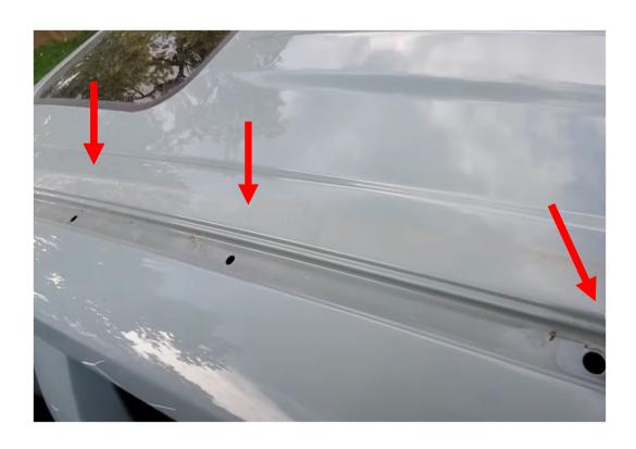
26. To affix the roof rails to the RAV4, Toyota uses a retainer clip at the points above the RAV4's A-pillar and C-pillar. Prior to September 2021, the retainer clip was identified as Toyota Part No. 6345142010. An image from the installation instructions for the roof rails is below.
