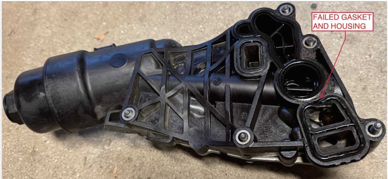
FIGURE 1: CLASS ENGINE OIL FILTER HOUSING FAILURE
