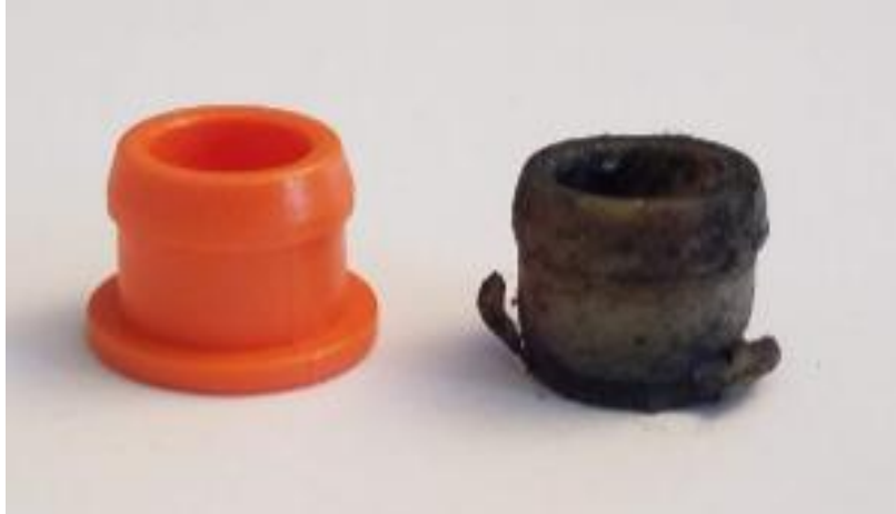
New Defective Bushing (left); Defective Bushing removed from a 2015 Ford Transit Connect after less than four years of use (right) 19
