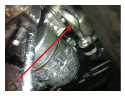
If the a/c line cracks, it may spray oil and refrigerant onto the a/c compressor, making the leak very hard to identify.
