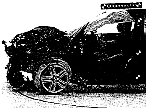
Small overlap front: — Driver-side —
