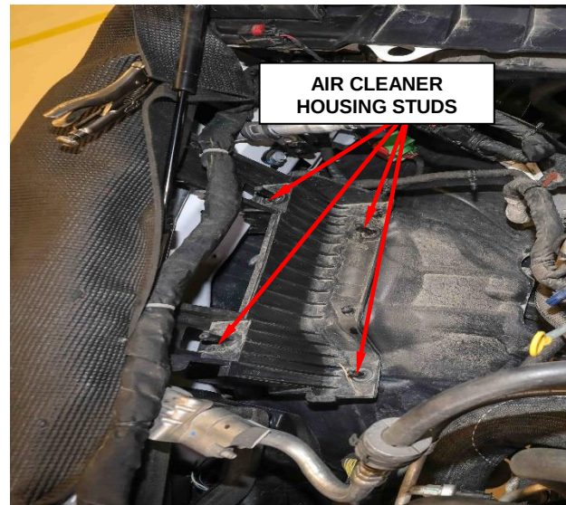
Figure 9 – Air Cleaner Housing Studs
