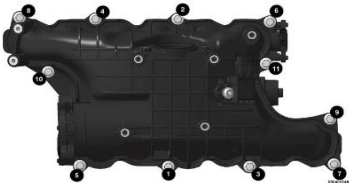
Figure 28 – Intake Bolts Tightening Sequence
